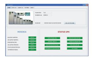
• An option of installing a LAN card with SNMP and HTTP protocols, which allows real-time monitoring of UPS devices anywhere in the country and abroad.
